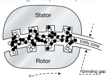
Due to the different taper of the splined conical face of the rotor and stator, a shrinking annular gap results in the direction toward the outlet cross-section. This is infinitely adjustable for all machines, even standard machines, via a locking collar and scale. High shear, compressive and friction forces work on the material particles for the desired result, determining grain size and throughput.
