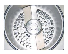
The diameter of the holes in the perforated disc is set depending on the base product and the desired grinding level. Related to this, the perforated discs are available with different hole diameters.
